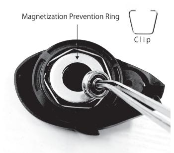
\* If it is difficult to pick out the magnetization prevention ring, insert a flat-blade screwdriver or other similar tools into a gap to pick it out. To avoid injury, don't use your nails as tools.
